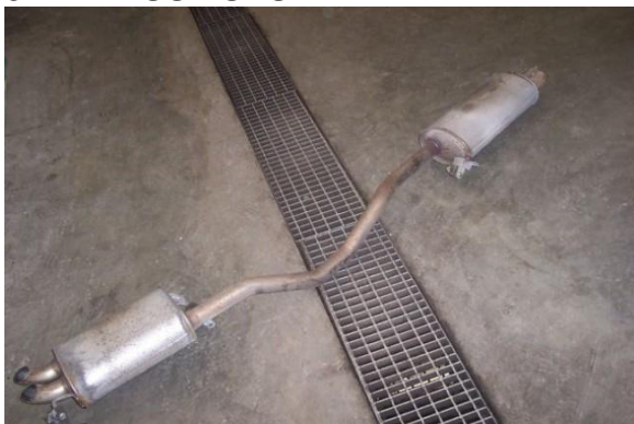
Dismount the original exhaust from the vehicle
