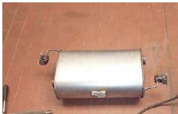
Cut the original pipes of the central exhaust
