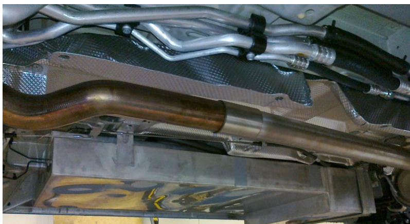
Connect the welded pipe to the back exhaust part
